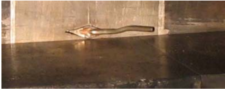
Figure 11. Moveable sidewall with diamond-shaped probe strut hole.
